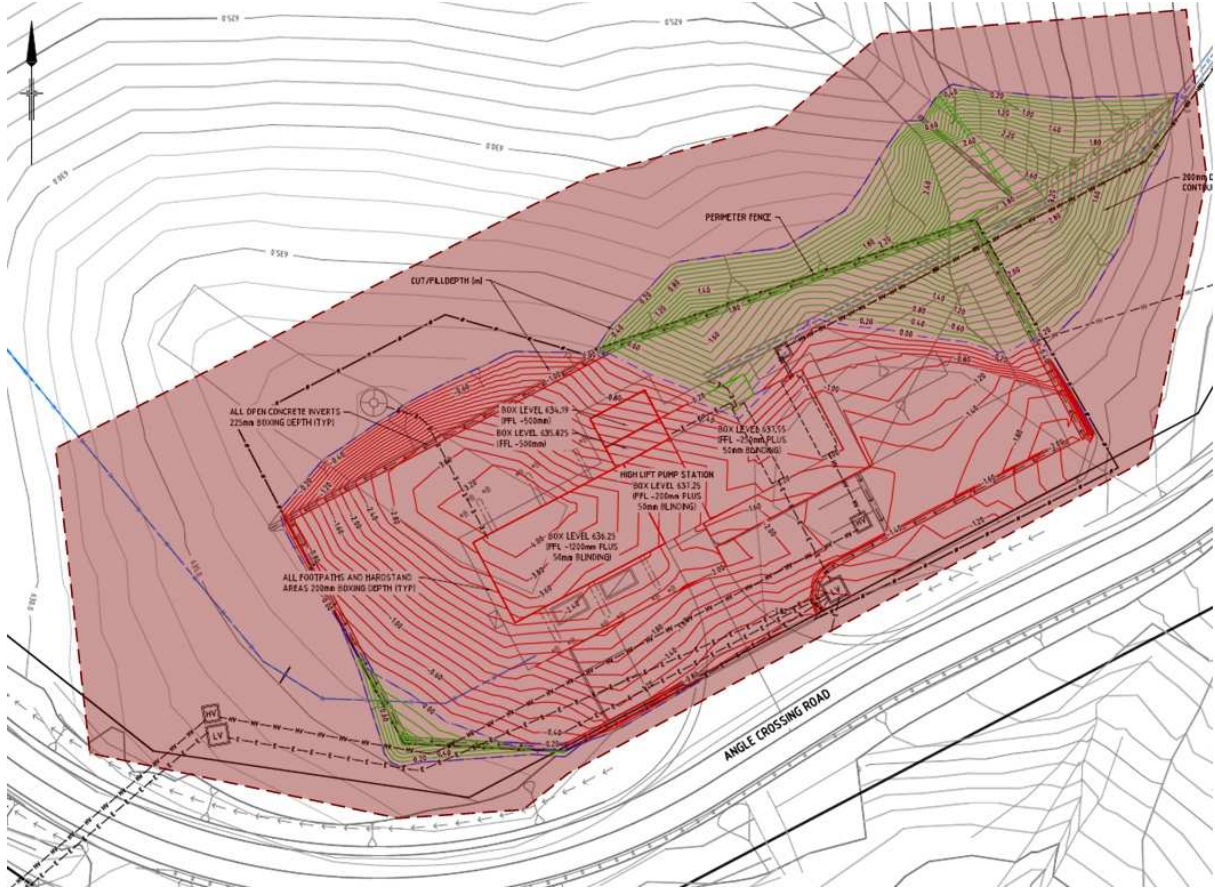
Figure 3.8 High Lift Pump Station Construction Boundary
