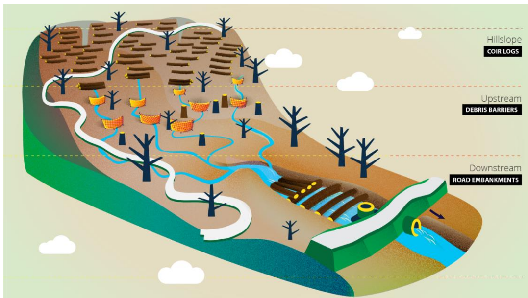
Figure 9. Techniques for erosion and sediment control in burned catchments. If appropriate, wood mulch or wood-shred can be used together with coir logs for a more intensive intervention strategy.
