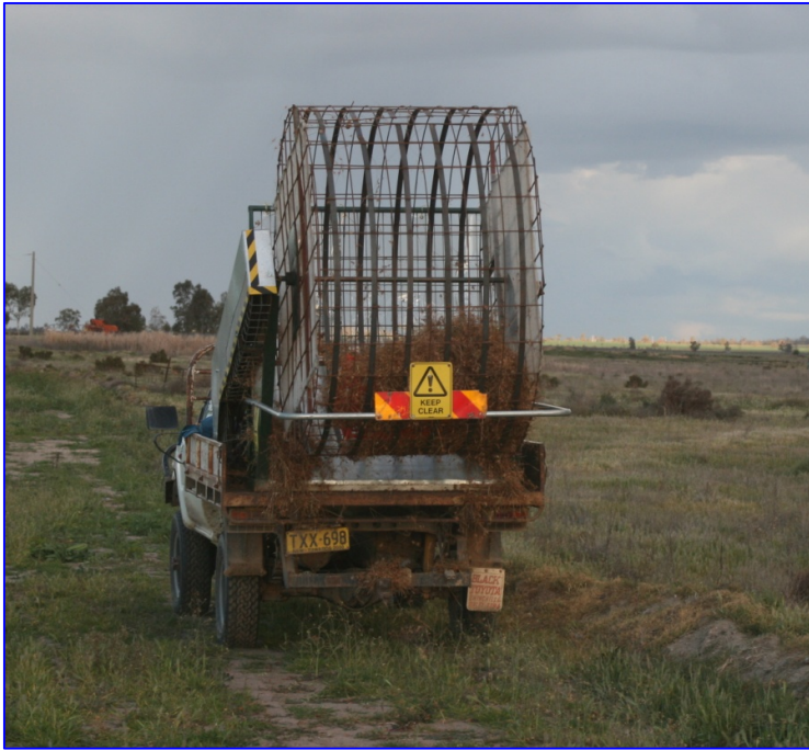
Figure 5.2 Purpose built native seed spreader – sowing being undertaken on soils typical to that found on the M2G pipeline
