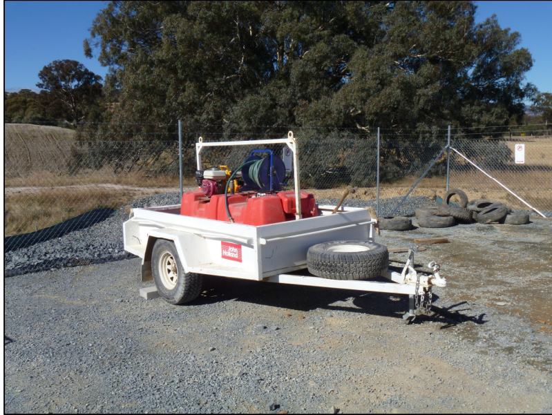
Figure 2.1 One of two weed wash trailers employed on the M2G project.
