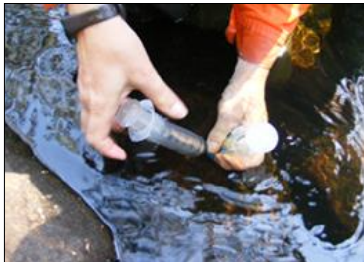
Plate 4. Periphyton sampler being used in the field
