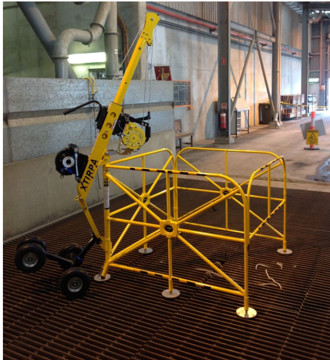
Fig. 5.7.4.3.1 Portable barrier with integrates davit (Image courtesy of SpanSet Australia Ltd)
