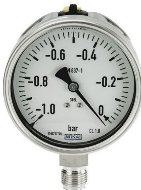
Fig. 6.1 Example of an acceptable analogue pressure gauge for a test pressure of -24 kPa (-0.24 bar)
