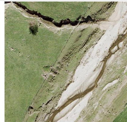
2017 Aerial of Naas River and tributary gully erosion and sediment build up, downstream of property access bridge.
