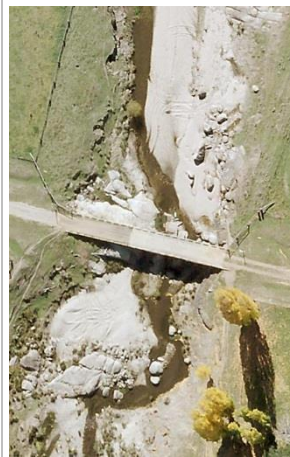
2017 Aerial of Naas River erosion and sediment deposition
