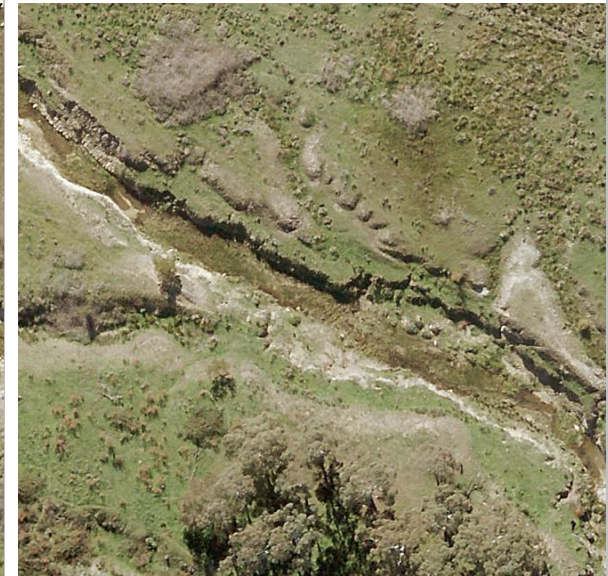
2017 aerial of bank erosion in Spring Station Creek downstream of the confluence with the gully
