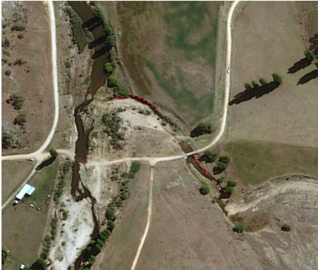
Composite aerial image of vertical banks present along Buchan Creek where bank stabilisation works are required
