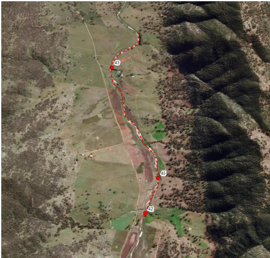
Aerial showing indicative location of several kilometres of active channel erosion
