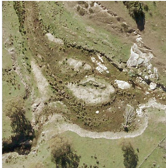
2017 aerial of bank erosion at confluence of Spring Station Creek and the gully
