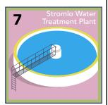
At Mount Stromlo Water Treatment Plant, the raw water goes through a process of filtration, disinfection by chlorination and UV treatment. This provides high quality drinking water to our suburban water reservoirs.
