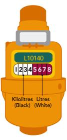
The black numbers show the kilolitres of water used by your home. This is used to calculate your water bill. The row of white numbers on the barrel show the litres and is used for monitoring usage.
