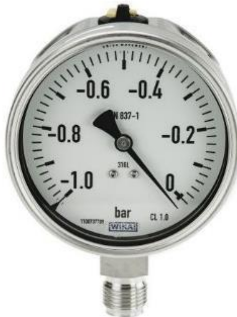
Fig. 12.2 An example of an acceptable analogue vacuum gauge for vacuum testing of sewer mains-to-tie pipe runs at -24 kPa (-0.24 bar)
