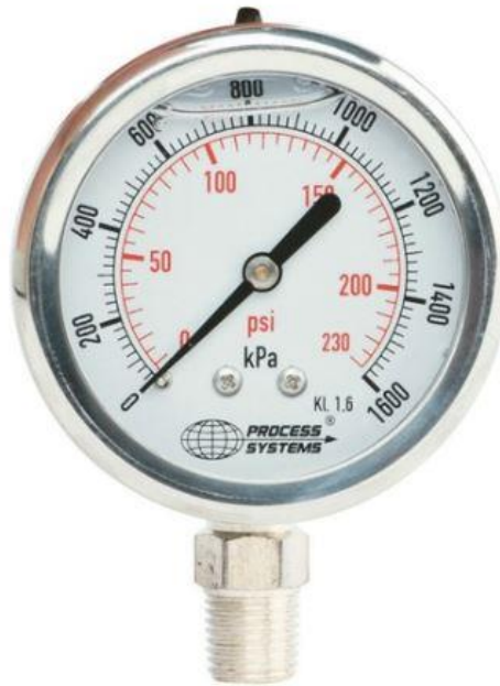
Fig. 12.1 An example of an acceptable analogue pressure gauge for hydrostatic testing of water mains-to-meter pipe runs at 1400 kPa (14 bar)
