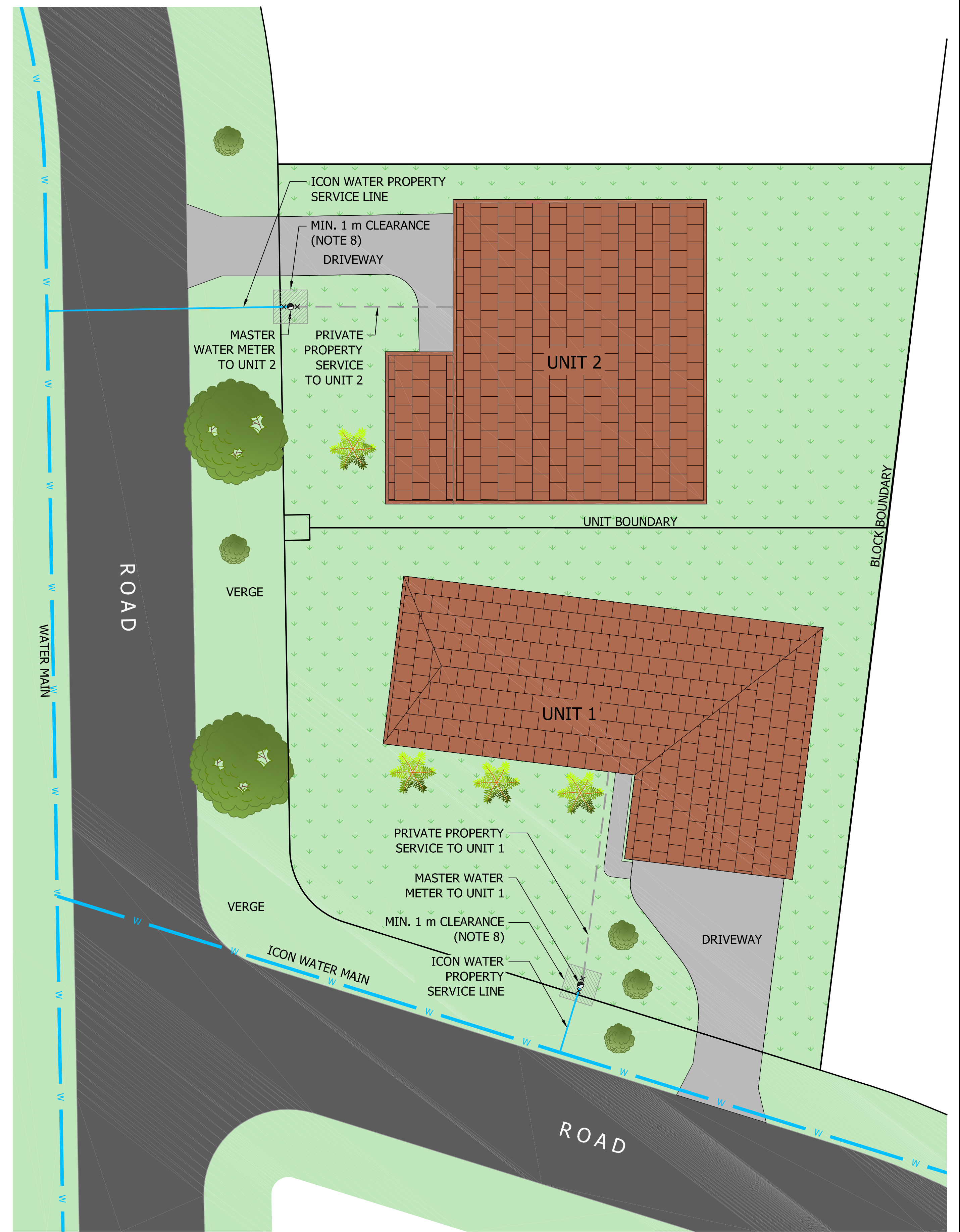
TYPICAL DUAL OCCUPANCY ARRANGEMENT FOR A PROPERTY WITH A WATER MAIN ON TWO BOUNDARIES (CORNER BLOCK)
