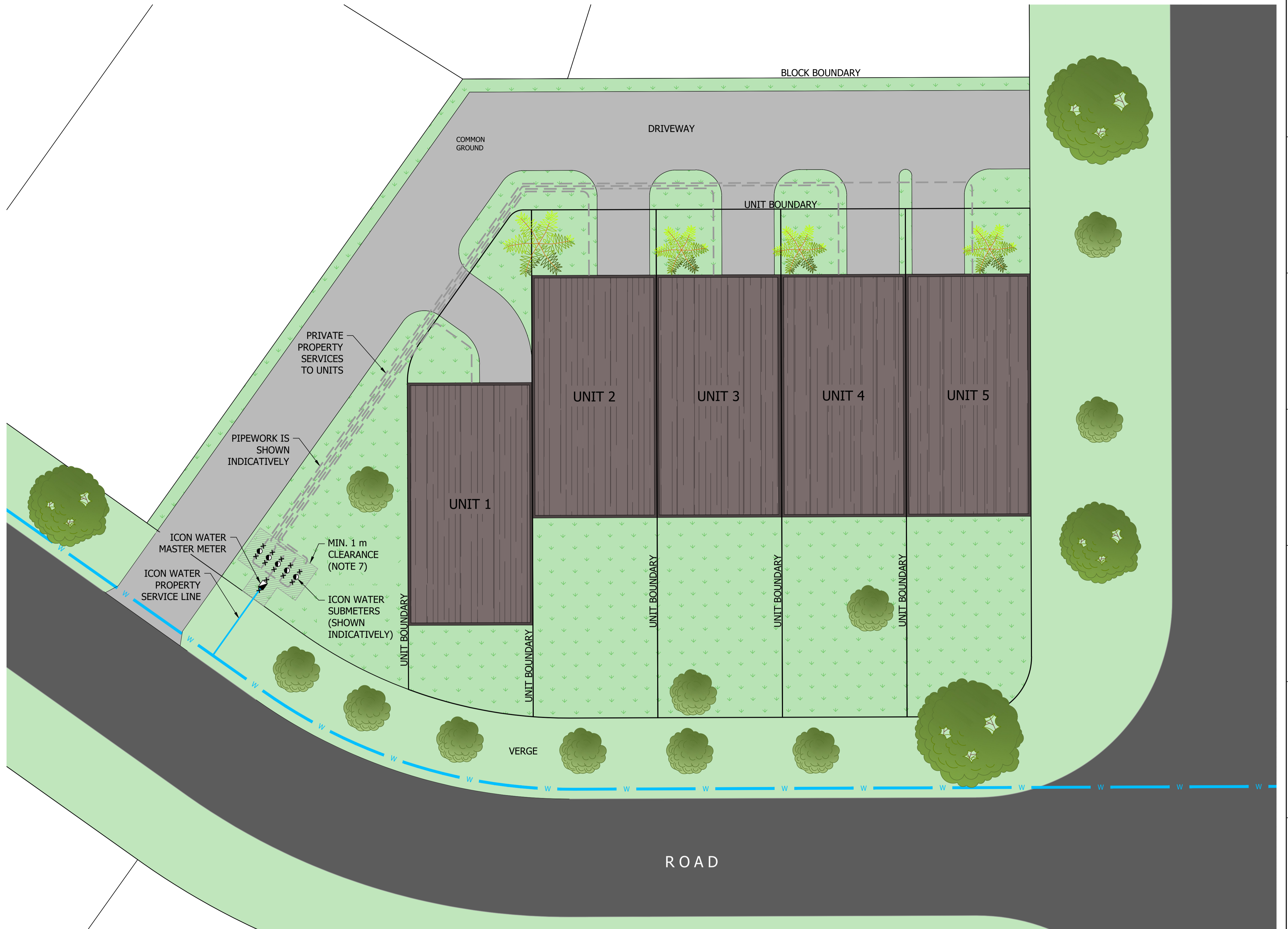
TYPICAL UNIT TITLE DEVELOPMENT FOR A PROPERTY THAT HAS 3 OR MORE UNITS WITH MASTER METER AT BOUNDARY AND SUBMETERS BELOW GROUND ADJACENT TO MASTER METER
